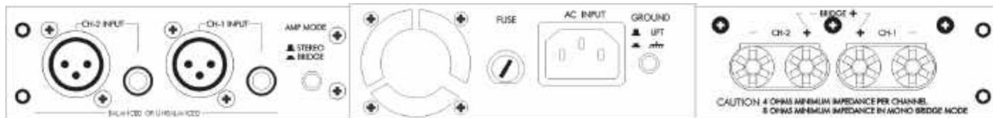
It is easy to interface the SLA-1 with a wide variety of equipment. All inputs and outputs are located on the rear panel. Standard ¼” and XLR inputs and binding post outputs make patching simple.
